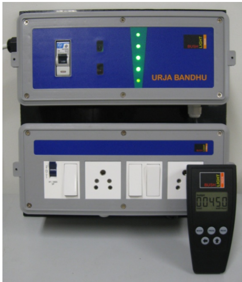
Image 1: The Urja Bandhu with integrated switchboard and remote programmer.
