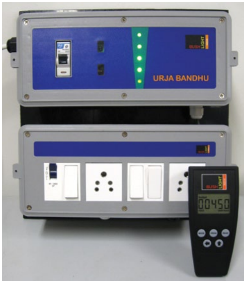
Urja Bandhu with programming module. The five lights count down as energy is used and thereby indicate the amount of budget available.
